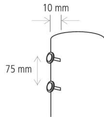
Thread the washers onto the nails or screws. Space the nails or screws 75 mm apart. Drive in the nails or screws, allowing them to protrude by 10 mm.
